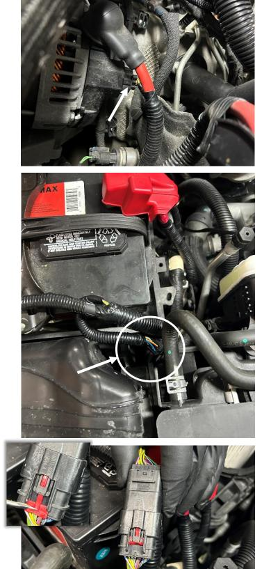
**STEP 7:** Connect the ends of the harness disconnected in the previous step to the passthrough connector on the Fleece Performance charging circuit harness. When both ends are connected, push the two red locking tabs into place.
